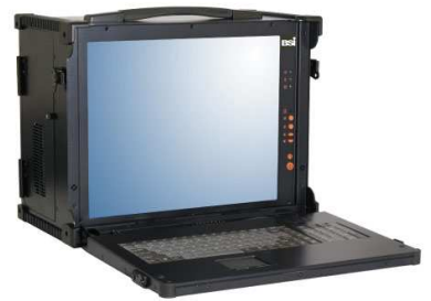
PA-PROW7-xxxx-00 Portable Workstation (7) PCI/PCIe Slots (4) Storage Bays 17" Sunlight readable Display
